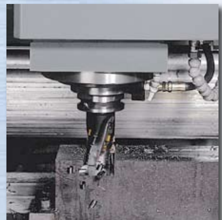
● Optimal Chip Removal (50#) End Milling
