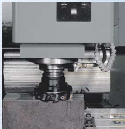
● Optimal Chip Removal (50#) Face Milling
