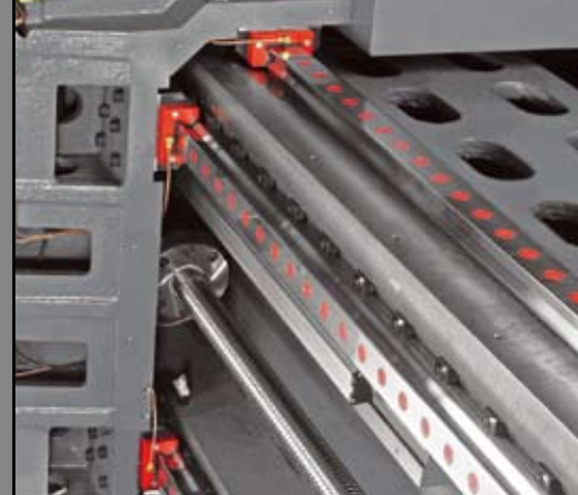
■ Horizontal and Vertical Support of the Headstock
