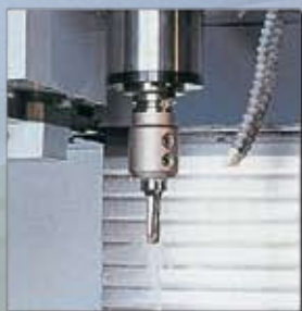
■ Coolant Through Spindle System
