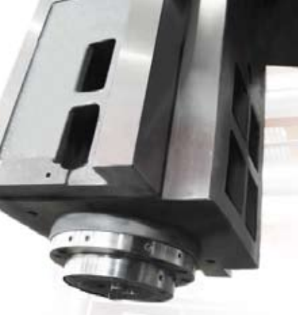
■ Hardened and Ground Box Guideway on Z-axis
